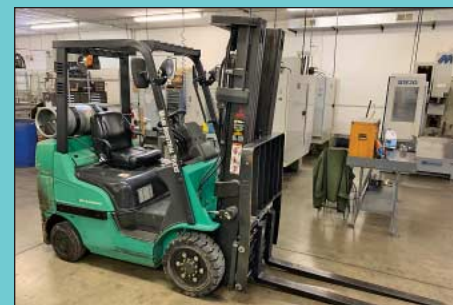
5,000 Lb. Mitsubishi Model FGC25N LP Gas Solid Tire Lift Truck
