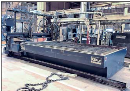
8' X 15' MG Plasma Table w/ Hyper-Therm Plasma Supply
