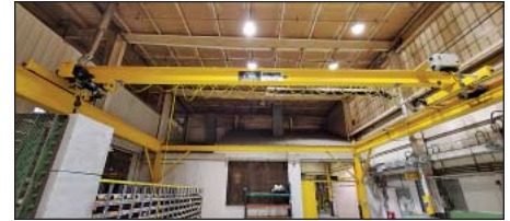
5-Ton x 32' Span Simmers Free-Standing Overhead Bridge Crane
