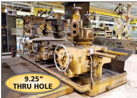
9.25" THRU HOLE Warner & Swasey No. 4A Turret Lathe w/ 9.25" Thru Hole
