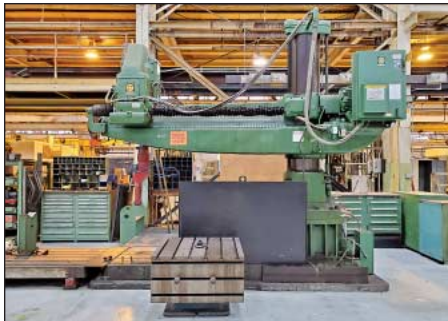
9' Arm x 15" Col. Cincinnati Bickford Radial Arm Drill
