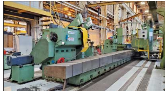
90" x 32' Safop Leonard Model 70/L-MC Large Capacity CNC Lathe with Milling & Y-Axis
