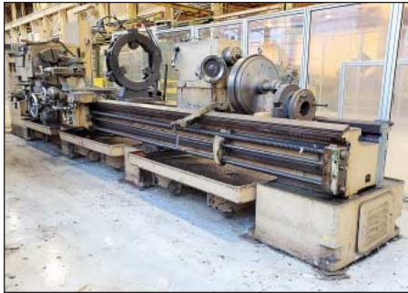
32" X 16' Leblond Model 3220-25 HD Engine Lathe
