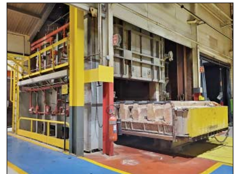
144" x 96" W x 68" H Dempsey Car Bottom Furnace to 1,800 Degree F
