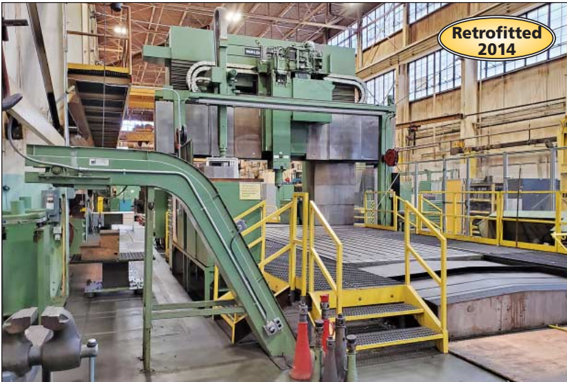
Waldrich Coburg Model PMC 3000 AT-F17 CNC Gantry Mill w/ 23' x 98" Table (Retrofitted Control 2014)
