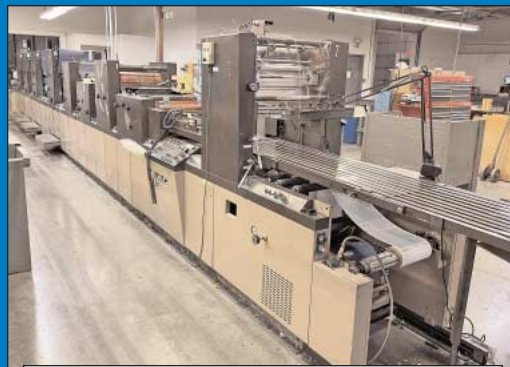
22" x 17" Didde 860 4-Color Web Press (Rebuilt 2001)
