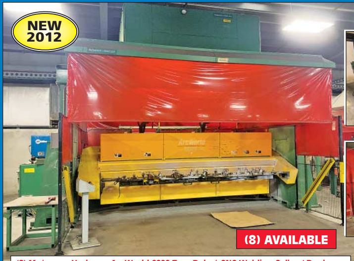
(8) Motoman Yaskawa ArcWorld 6200 Two-Robot CNC Welding Cell w/ Dual Headstock Tailstock Positioners
