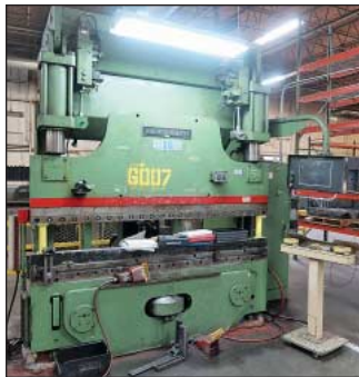
135 Ton x 8' Cincinnati 135AF x 6FT Autoform Six-Axis Press Brake w/ Crowning
