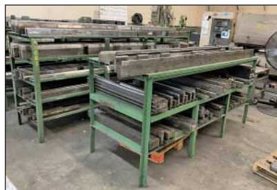
Large Quantity of Various Size & Style Press Brake Dies, Top, Bottom, V-Dies & Gooseneck
