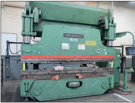
230 Ton x 12' Cincinnati 230AF x 10FT Autoform Three-Axis Press Brake w/ Crowning
