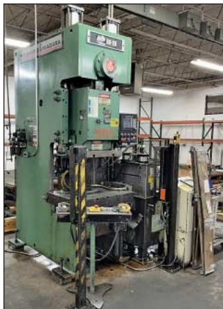
(2) 88 Ton Clearing Niagara Model BN-80-I Gap Frame Presses
