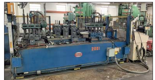
Yoder 3-Stand Rollformer w/ (2) 18" x 20" Pneumatic Cut-Offs
