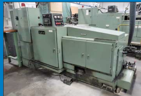
Asahi Okuma Model AOT-6XL High Speed Long Stroke 2-Die 2-Blow Cold Header
