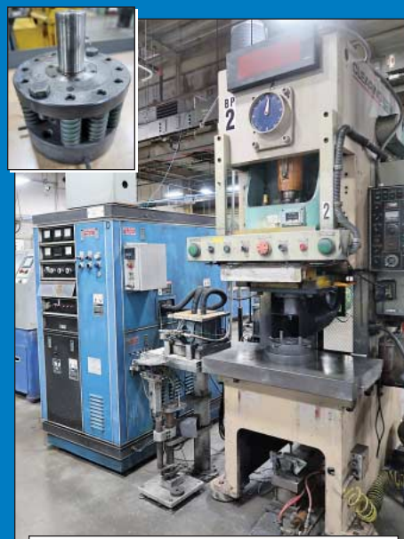
88-Ton & 66-Ton Seyi Clearing Presses Converted to Forge 12-Point Aircraft Engine Bolts
