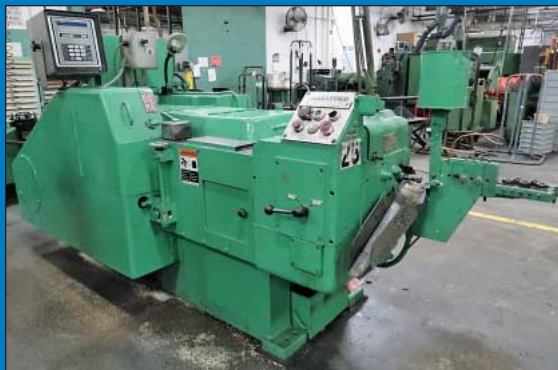
Hartford Model 3-500 High Speed Single Stroke Solid Die Long Stroke Cold Header
