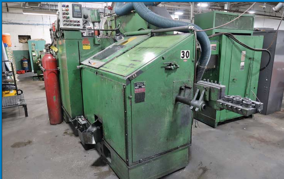
National Model 56HSLs High Speed DSSD Cold Header Converted to Run Aerospace Fasteners Using Induction Heat
