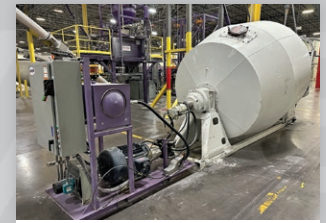
(10) Skid Mount 50-HP Concrete Truck Style Mixers
