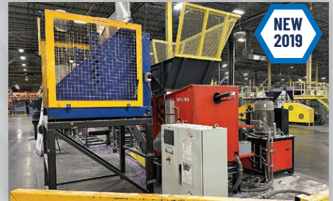
60-HP Weima Single Shaft Shredder
