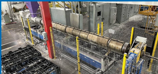
(6) 6" x 280" Barrel Single Screw Extruders, 300-HP and 450-KW Drives
