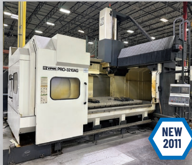
Mighty Viper Model PRO-3210AG Bridge Type CNC VMC
