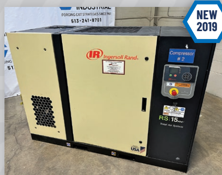
(2) 20 HP Ingersoll Rand RS15NE-A135-TAS Air Compressors
