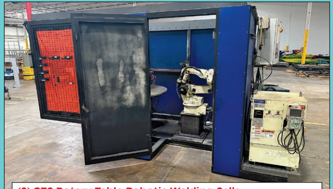
(2) OTC Rotary Table Robotic Welding Cells
