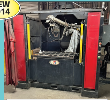
(2) Fanuc Lincoln Pick and Place Robotic Welding Cells
