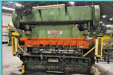
**Mechanical Press Brakes to 150 Ton x 10'**
