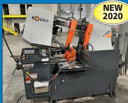
**18" x 18" Cosen C460NC-CE CNC Horizontal Band Saw**
