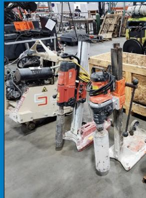
Core Drills and Concrete Saw
