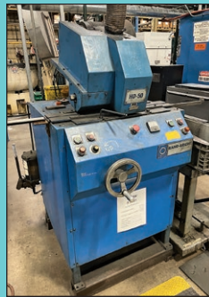
(2) 80 KW Tocco Toccoatron Induction Rod Heaters w/ Randbright Polishers
