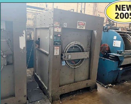
(2) 130 Lb. Milnor Model 42026X7J Batch Washer Extractors
