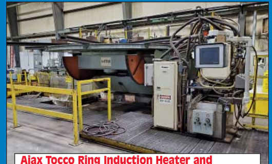
Ajax Tocco Ring Induction Heater and 74,000 Lb. Aronson Weld Positioner
