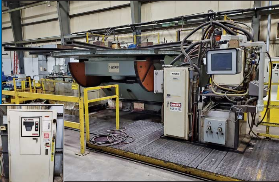
Ajax Tocco Ring Induction Heater and 74,000 Lb. Aronson Weld Positioner
