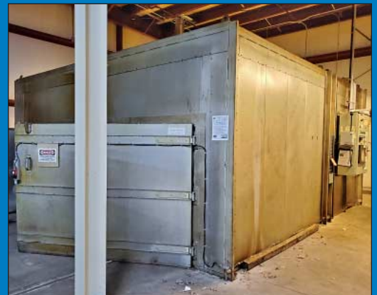
16' x 15' x 4' High Natural Gas Fired Tempering Oven
