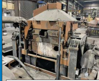
(6) 12,000 Lb. Ajax Magnethermic TET 500-KW Induction Melt Furnaces
