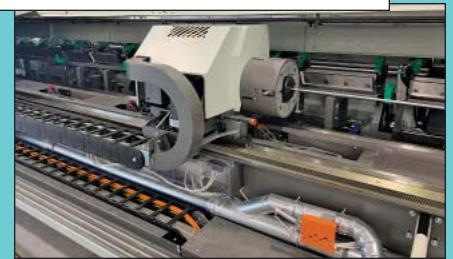
(3) 4,000 Watt BLM Group Model Lasertube LT7 Fiber Optic Tube Laser w/ Dust Collector & Chiller
