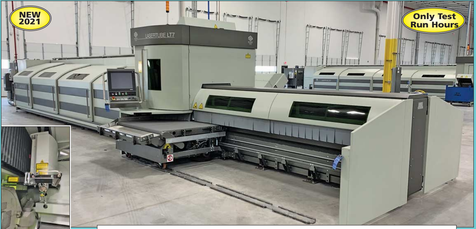
(3) 4,000 Watt BLM Group Model Lasertube LT7 Fiber Optic Tube Laser w/ Dust Collector & Chiller
