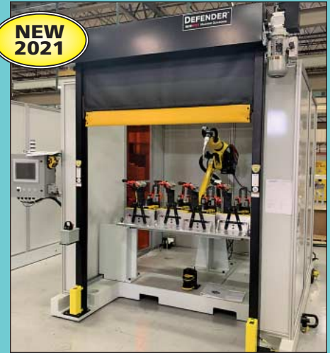
Artiflex Robotic Welding Cell #5915-4100 with (1) Fanuc Arcmate 100iD Six-Axis Robot
