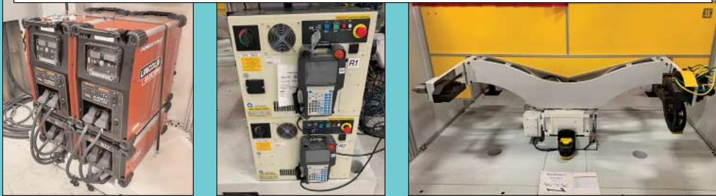
(8) Artiflex Two-Station Robotic Welding Cells w/ (2) Fanuc Arcmate 100iD Six-Axis Robots, (2) 30" X 48" Trunnion Tables, & (2) Lincoln R450 Power Welders (New 2021)
