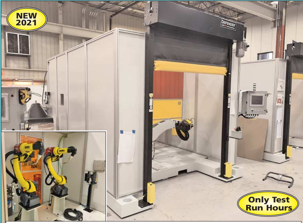
(8) Artiflex Two-Station Robotic Welding Cells w/ (2) Fanuc Arcmate 100iD Six-Axis Robots, (2) 30" X 48" Trunnion Tables, & (2) Lincoln R450 Power Welders (New 2021)
