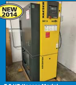
7.5 HP Kaeser Model Aircenter SM 7.5 Packaged Compressor System
