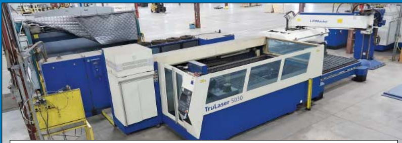
6,000-Watt and 5,000-Watt Trumpf Trulaser 5030 CO2 Lasers w/ Lift Masters
