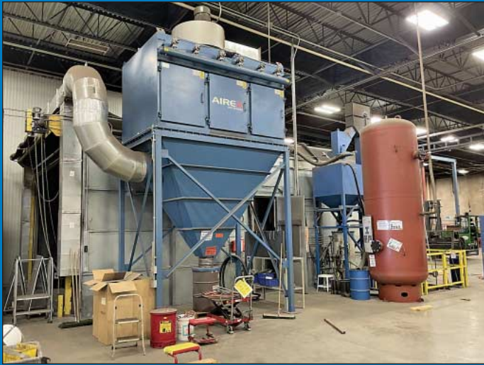
16' x 24' x 11' H Drive-In Blast Room, Dust Collector and Reclaim
