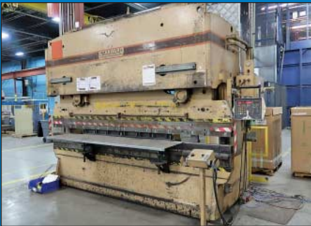
250 Ton x 12' Standard Hydraulic Press Brake
