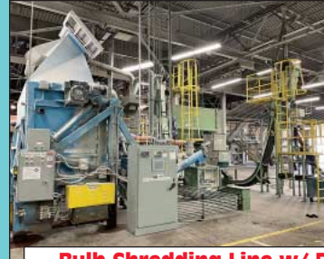
Bulb Shredding Line w/ Eriez / Bunting Units, Dumper, Crush, Dust Collection
