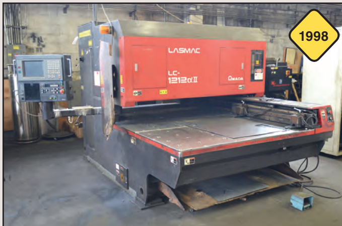
1.5Kw Amada LC1212A2 Pulsar Hybrid Laser
