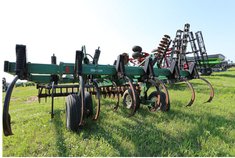
Glenco 14' Soil Saver with Spring Trips. Purchased New 1/18/2011. 5 shanks, deep rippers front, 7 shanks behind. Serial #2701
