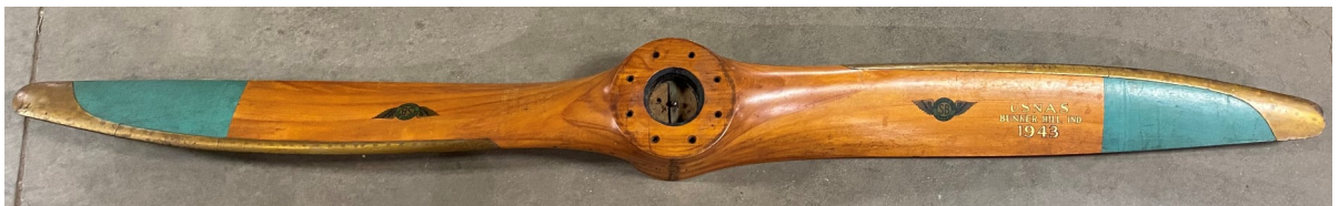
8' 1943 Sensenich Bros, Lititz, PA. USNAS, Bunker Hill, IND. PT-17 Airplane; R-670-5 Engine; 220 HP; 2100 RPM. Part No. 42K19593; SER No. 52281.
