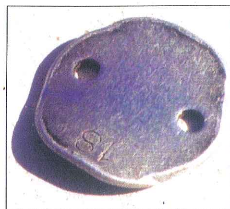
I removed the manifold and found a carburetor throttle plate floating around inside.
