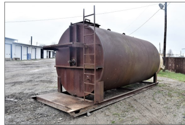
6000 Gallon mixing tank
