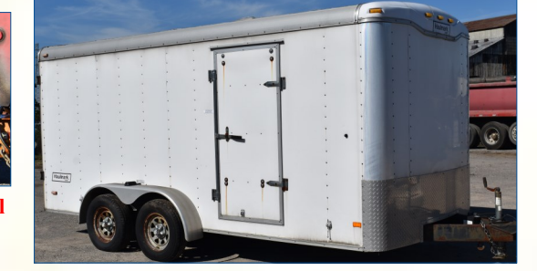
144. 2004 Haulmark 16' enclosed trailer. 7000 lb GVW, 5 lug tires, cargo door 72" door height, 6" door width.
