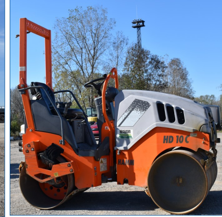
102. 2016 Hamm HD 10C Compactor Roller. 39" wide, 24" diameter; offset roller, smooth drum tandem vibratory roller, 1900 hours.
