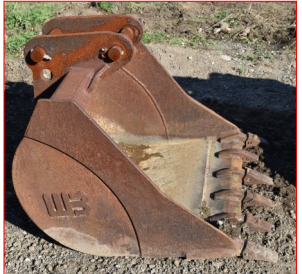
172. WB 36" Excavator bucket, 8" pin spacing, 2 1/4" pin, 12" width Fits Yanmar Excavator.
