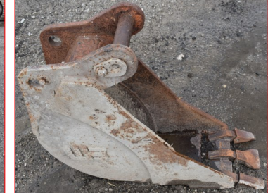
184. WB Backhoe trench bucket, 2 1/8" front pin, 2" back pine, 12" in between centers, 8" spacing.
