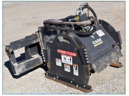
130. 2015 Case 30" Asphalt Cold Planer Skid Mount. Hydraulic adjustment, tilt & angle and side shift. Clean
