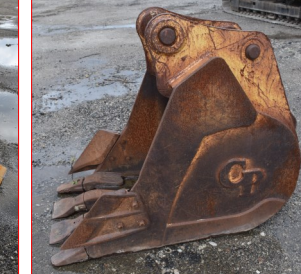
182. GP Excavator bucket, 30" wide, 44" tall, 5' depth, 3 1/8" pin, 18 1/2" in between centers, 12" spacing
