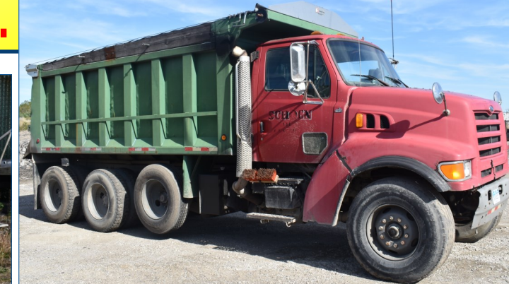
116. 1998 Ford T-91 tandem axle dump truck, with drop axle, 425/65R 22.5 fronts, 11R 22.5 rears, 16' dump bed, hand crank tarp, Eaton Fuller 8 speed, CAT diesel. 1 Owner
