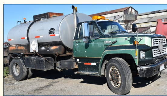
154. 1992 Ford F800 w/Etnyre Asphalt Distributor topser series 2000, 12' spray boom, 2000 gallon tank, propane fired burner, spray wand, 5 speed w/2 speed rear, 11R 22.5 tires, 354,000 miles.
