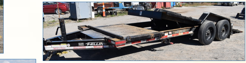
140. 2016 Felling FT-15 IT-1 tandem tilt trailer. 18,000 lbs GVW, 8 lug 215/75R 17.5, 20" wide ramp, 5'11" in between
