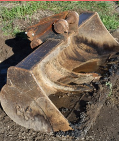
176. BK 60" Ditch Bucket, 8" pin spacing, 2 1/4" pin, 12" width Fits Yanmar Excavator
