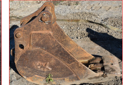
164. BK 12" trench bucket, 8" pin spacing, 2 1/4" pin, fits Yanmar Excavator
