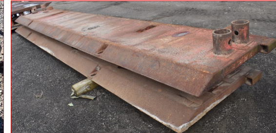
198. 24' x 4' Pro-Tec trench box, with paperwork and OSHA Certification. 4" double wall
