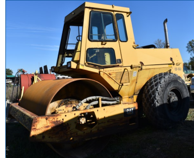
113. 1989 CAT CS-553 vibrating compactor, smooth drum, 7' wide x 60" drum, 5500 hrs, no front or rear glass, runs & drives Vibratory.
