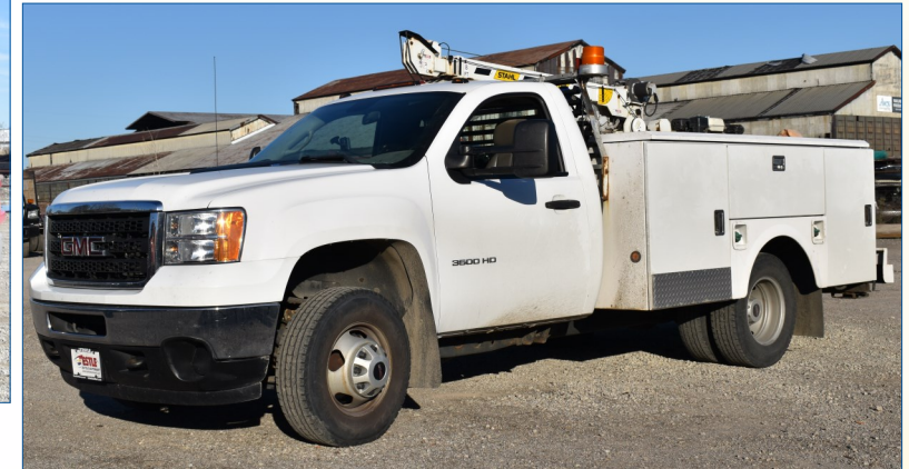
122. 2011 GMC 3500 4x4 service truck, Duramax 6.6 diesel, 235/80R 17 tires, 82,000 miles, automatic Allison has Stahl 9 1/2' service body & Stahl 4000 CRX 16' telescopic boom, rear stabilizer 90 gallon fuel tank.
