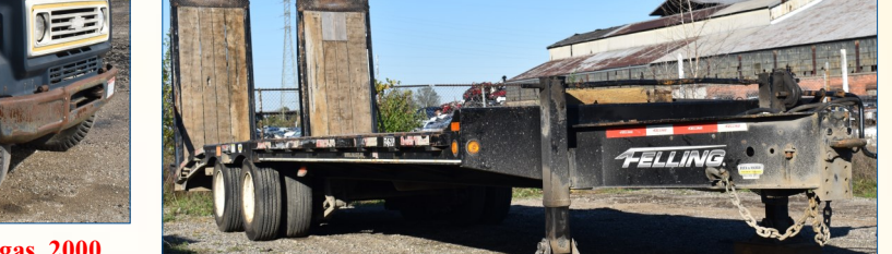
136. 2017 Felling FT-45-2LP tandem dual trailer, air brake, air flip up ramps, 235-75R 17.5 8 lug tires, rub rail & chain box, 22' + 6' beaver, 8'6" wide, 7'6" x 37" wide ramps. Used to haul LeeBoy 8520 B paver with, Hamm 14 roller.
