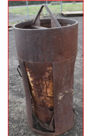
196. 1 Yard homemade concrete pouring
