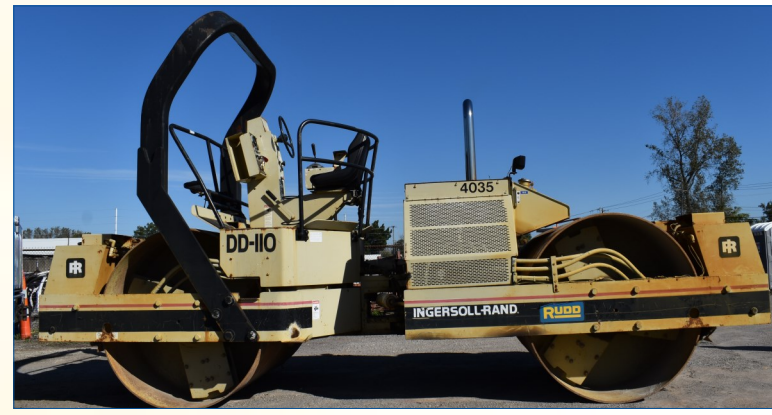
105. 1996 Ingersoll Rand DD-110 Compactor Roller. 6'6" wide x 53 1/2" smooth drum, 5230 Hours, Vibratory compactor.
