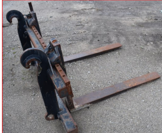
120. Wheel loader 4" pallet fork, 39 1/2" wide in between center, 24" spacing
