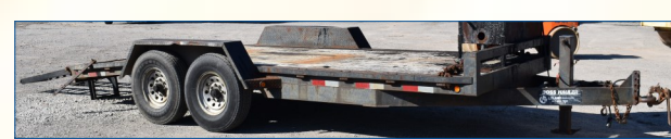
142. 2003 Leland 18' tandem trailer w/4' beaver, 5' flip up ramps, LT 235/85R 16 tires, 8 lug, electric brake, 6'8" in between fenders.
