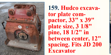
159. Hudco excavator plate compactor, 33" x 39" plate size, 3 1/8" pine, 18 1/2" in between center, 12" spacing. Fits JD 200 Excavator
