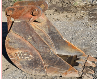
168. WB 18" Excavator bucket, 8" pin spacing, 2 1/4" pin, 12" width Fits Yanmar Excavator.
