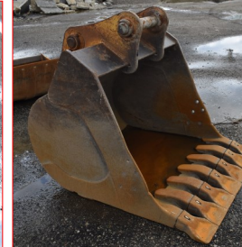
180. BK Excavator bucket, 48" wide, 44" tall, 5' depth, 3 1/8" pin, 18 1/2" in between centers, 12" spacing
