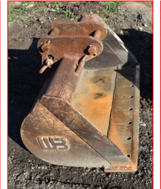
174. WB 48" ditch bucket, 8" pin spacing, 2 1/4" pin, 12" width Fits Yanmar Excavator
