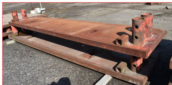
202. 16' x 4' Pro-Tec trench box, with paperwork and OSHA Certification. 4" double wall.
