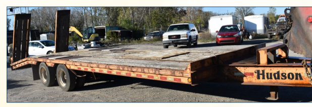
138. 2007 Hudson 20 ton trailer 22' +6' Beaver Tail. Model HTD18A 48,640 GVW tandem dual 215/75R 17.5 tires, 8 lug, air brakes, 8'6" wide, 8'10" flip up ramps, rub rail, LED lights.
