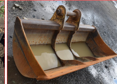
178. 72" Ditch grading bucket, 3 1/8" pin, 18 1/2" in between centers, 12" spacing. Fits JD 200 Excavator.
