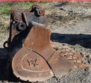
170. BK 30" Excavator bucket, 8" pin spacing, 2 1/4" pin, 12" width Fits Yanmar Excavator
