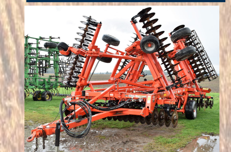
24 2015 Kuhn Krause 30' Excelerator 8000, Vertical Till 30' working width; 8" disc spacing; LED lights; Adjustable gangs; walking tandems
