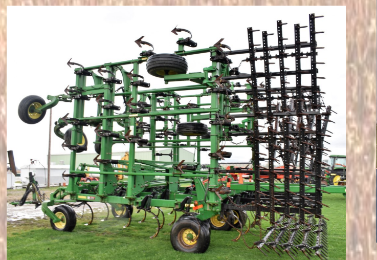
25 John Deere 48' 220 Field Cultivator, Walking tandems, Floating Hitch, 48' working width, 5 Bar harrow clod buster
