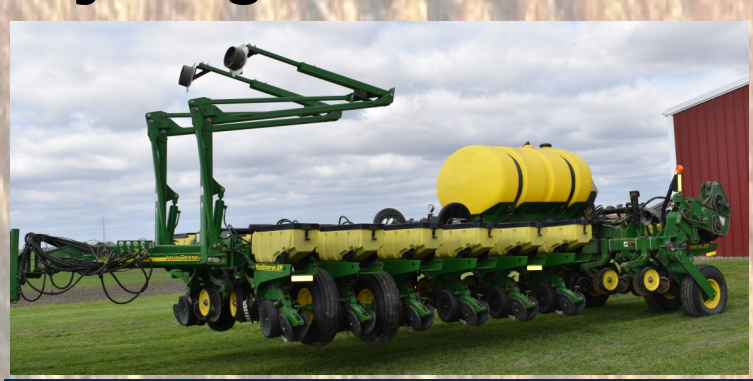
16 2008 John Deere 1770NT 16 row planter, MaxEmerge XP 600 gallon liquid tank, 30" row spacing, Martin free flowing spike tooth openers, rear hitch & light hookup with cab controller; Pneumatic down pressure, Delivery date November 2008
