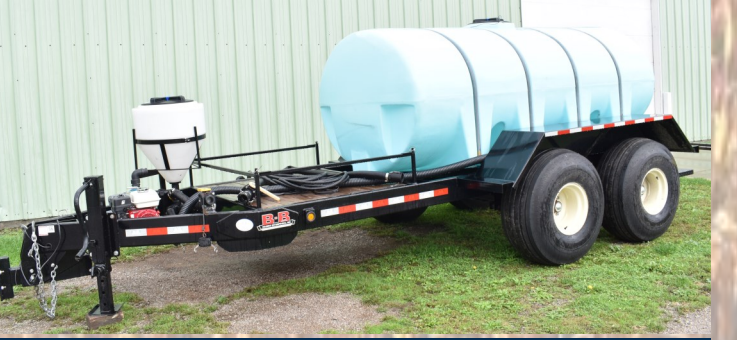
18 2016 Behnke 2000 gallon tank trailer, 18,000 GVW, Used for fertilizer, 2" quick coupler Hoses, Honda Pump, Pin Hitch, 7 way flat light plug, 16.5L-16 tires, LED Lights, 30 gallon Induction tank. Super clean like new!
