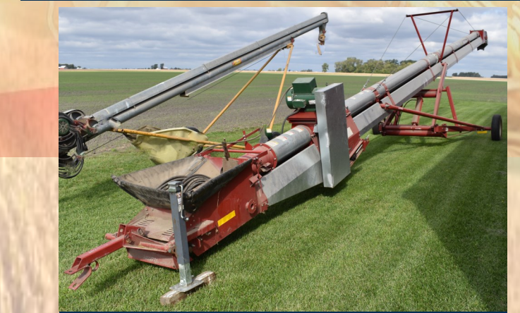
35 Hutchinson 10'x62' conveyor, with 10 hp Dayton 1ph 230V motor with lead cord, hydraulic lift, serial #916076
