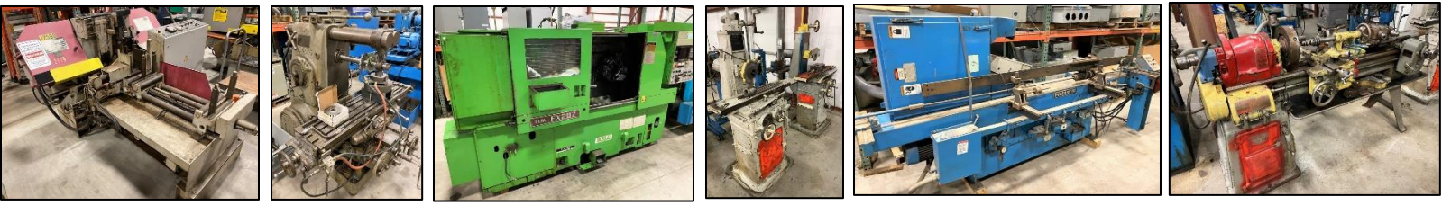
LEFT-RIGHT: Behringer HBP260A 11.8" x 10.2" Automatic Horizontal metal cutting bandsaw; Milwaukee model K horizontal mill; IkeGai FX20Z CWC turning center lathe; Brown & Sharp #2 & #2b surface grinders; South Bend CL8145 engine lathe
