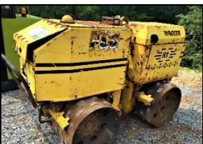
Wacker RT trench compactor
