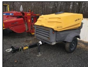
Atlas Copco Air Compressor
