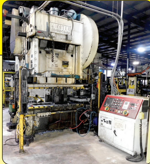
Minster Model G2-150-72-30 Gap Frame Press
