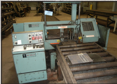
W.F. WELLS Model W-10-2; 10' x 17" Semi-Automatic Twin Post Horizontal Band Saw; In and Out Conveyor
