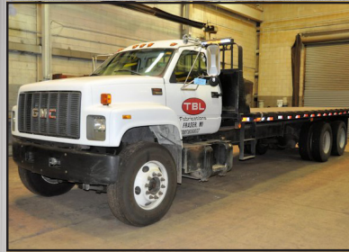
1996 GMC Model C7500; Tandem Axle Quad Wheeled 8' x 24' Stake Body Truck; Diesel Engine, Air Brakes
