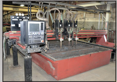
MESSER APOLLO/HSG; 9' x 24' CNC Plasma Cutting System 1 Plasma, 4 Oxy (Rebuilt Approx 5 Years Ago)
