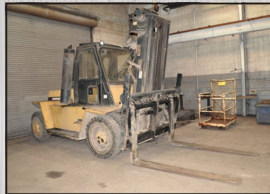
CATERPILLAR Model V225B; 22,500-Lbs. X 218" Lift Capacity Diesel Fork Lift Truck; 7' Forks
