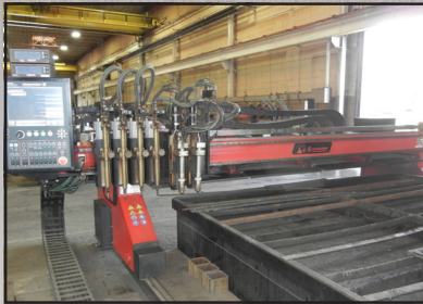
CUTTING SYSTEMS KODIAK 10' x 50' High Def CNC Plasma Cutting System (2014) 2 Plasma 4 Oxy, Burney CNC Control, (Approx. 500 Total Hours on Machine).
