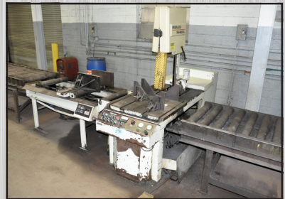
PEERLESS Model VB-1820XLA; 18" x 20" Automatic Tilt Frame Vertical Band Saw; w/ In / Out Conveyors
