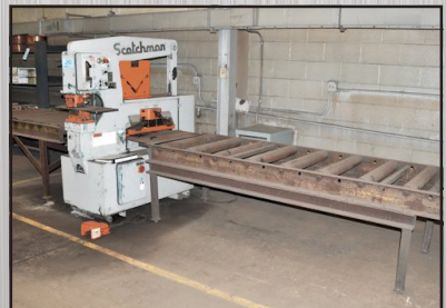
SCOTCHMAN 6509-24M; 65-Ton Capacity Hyd. Ironworker; (2004), 24" Shear, 6" x 6" Angle, Conveyors
