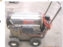
Diesel fired hot water heater for power washer,
