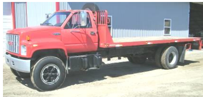
1992 GMC Topkick #3116 cat. Dsl, 5 spd, man. w/Hi-Low rear end brakes, Schwartz 21' roll back tilt w/2' endgate, shows 32,245 mi.- only 1689 hr on engine, Note: formerly a MI DNR truck for hauling fire bulldozer,
