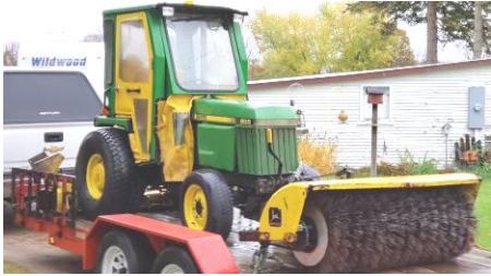
John Deere 955 dsl, hydro stat. 4 wd tractor, canvas cab has front mt 246 sweeper and 72" belly mower deck,
