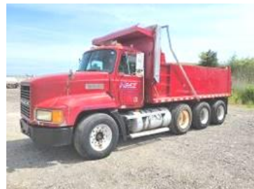
1993 MACK tri axle, 16' dump truck, mdl ch613, 8 spd, hi-low trans, EM7-300 Mack, 50K on motor, 300k mi,
