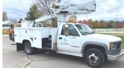
2001 GMC 3500 HD cab & chassis, 6.5 turbo dsl. Autotrans, dual r/r wheels, w/13' tool box bed, 400 lbs. Versal lift bucket, Aerial truck, Insulated, 20,789 mi, (passed insp. 5/25/21)
