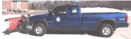
2004 Chevrolet 2500HD, 4x4, ext. cab, long box p/u, w/western plow, 153,776 mi, (trans slips in 4wd when plowing)
