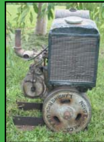
rare Nova AG upright w/ cooling radiator
