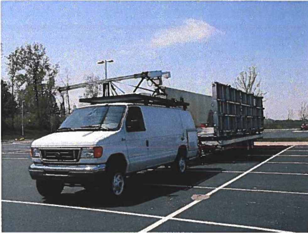
Range in Transport Configuration attached to Antenna Van
