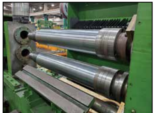
LIGHT GAUGE SLITTING LINE: STAMCO - Pancake Cuts, Non-Plate Strip, .010" - .040" Gauge, .625" - 25.5" Width, 450 FMP, Payoff Arbor - 16" - 20" @16,000-lb., Take-up Arbor - 12.0", 16.0", 20.0" • 520 PIW, PRO-ECO 4 Turnstile Coil Holder, Entry Coil Cart on Track, Payoff Reel Pusher/Tensioner, HORSBURGH & SCOTT Expanded Mandrel De-Coil Reel, STAMCO Breaker, Pinch & Bridle Roll Machines, STAMCO Crop Shear, Out Feed Chip Conveyor, (2) STAMCO Slitting Heads, Tension Roll, Stripper Plate, Loop Tables, Coiling End Reel, End Line Coil Transfer Carriage on Track, (3) Operator Stations, ABB Centerline MCC's, Breaker Cabinet, (5) Transformers, ROCKWELL Automation Drives
