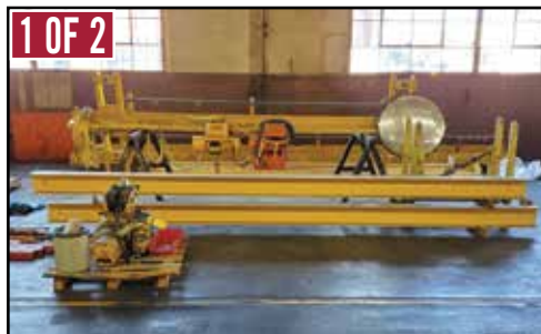
PEC 1/2-Ton x 14' Span Free-standing Bridge Crane
