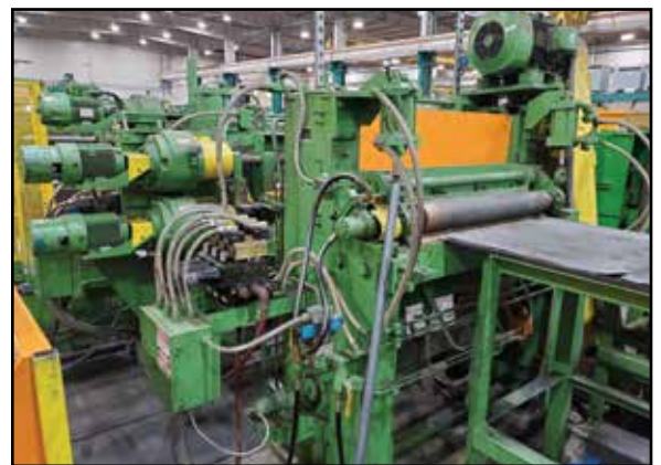
HEAVY GAUGE SLITTING LINE: STAMCO - Pancake Cuts, Non-Plate Strip, .040" - .150" Gauge, .460" - 25.5" Width, 450 FMP, Payoff Arbor - 16" - 20" @16,000-lb., Take-up Arbor - 12.0", 16.0", 20.0" • 520 PIW, PRO-ECO 4 Turnstile Coil Holder, Entry Coil Cart on Track, Payoff Reel Pusher/Tensioner, HORSBURGH & SCOTT Expanded Mandrel De-Coil Reel, STAMCO Breaker, Pinch & Bridle Roll Machines, STAMCO Crop Shear, Out Feed Chip Conveyor, (2) STAMCO Slitting Heads, Tension Roll, Stripper Plate, Loop Tables, Expanding Mandrel Coiling Reel, End Line Coil Transfer Carriage on Track, (3) Operator Stations, ABB Centerline MCC's, Breaker Cabinet, (5) Transformers, ROCKWELL Automation Drives
