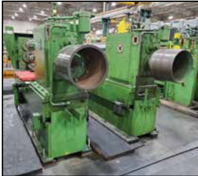
HEAVY GAUGE SLITTING LINE: STAMCO - Pancake Cuts, Non-Plate Strip, .040" - .150" Gauge, .460" - 25.5" Width, 450 FMP, Payoff Arbor - 16" - 20" @16,000-lb., Take-up Arbor - 12.0", 16.0", 20.0" • 520 PIW, PRO-ECO 4 Turnstile Coil Holder, Entry Coil Cart on Track, Payoff Reel Pusher/Tensioner, HORSBURGH & SCOTT Expanded Mandrel De-Coil Reel, STAMCO Breaker, Pinch & Bridle Roll Machines, STAMCO Crop Shear, Out Feed Chip Conveyor, (2) STAMCO Slitting Heads, Tension Roll, Stripper Plate, Loop Tables, Expanding Mandrel Coiling Reel, End Line Coil Transfer Carriage on Track, (3) Operator Stations, ABB Centerline MCC's, Breaker Cabinet, (5) Transformers, ROCKWELL Automation Drives
