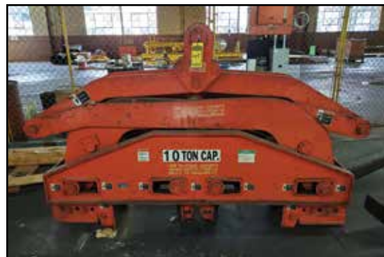
RUSHMAN 10-Ton Man Saver Scissor Type Coil Lift
