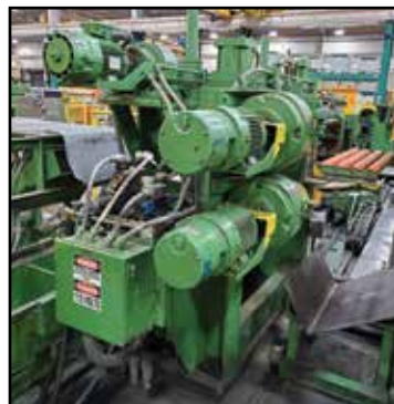
LIGHT GAUGE SLITTING LINE: STAMCO - Pancake Cuts, Non-Plate Strip, .010" - .040" Gauge, .625" - 25.5" Width, 450 FMP, Payoff Arbor - 16" - 20" @16,000-lb., Take-up Arbor - 12.0", 16.0", 20.0" • 520 PIW, PRO-ECO 4 Turnstile Coil Holder, Entry Coil Cart on Track, Payoff Reel Pusher/Tensioner, HORSBURGH & SCOTT Expanded Mandrel De-Coil Reel, STAMCO Breaker, Pinch & Bridle Roll Machines, STAMCO Crop Shear, Out Feed Chip Conveyor, (2) STAMCO Slitting Heads, Tension Roll, Stripper Plate, Loop Tables, Coiling End Reel, End Line Coil Transfer Carriage on Track, (3) Operator Stations, ABB Centerline MCC's, Breaker Cabinet, (5) Transformers, ROCKWELL Automation Drives
