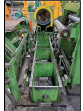
HEAVY GAUGE SLITTING LINE: STAMCO - Pancake Cuts, Non-Plate Strip, .040" - .150" Gauge, .460" - 25.5" Width, 450 FMP, Payoff Arbor - 16" - 20" @16,000-lb., Take-up Arbor - 12.0", 16.0", 20.0" • 520 PIW, PRO-ECO 4 Turnstile Coil Holder, Entry Coil Cart on Track, Payoff Reel Pusher/Tensioner, HORSBURGH & SCOTT Expanded Mandrel De-Coil Reel, STAMCO Breaker, Pinch & Bridle Roll Machines, STAMCO Crop Shear, Out Feed Chip Conveyor, (2) STAMCO Slitting Heads, Tension Roll, Stripper Plate, Loop Tables, Expanding Mandrel Coiling Reel, End Line Coil Transfer Carriage on Track, (3) Operator Stations, ABB Centerline MCC's, Breaker Cabinet, (5) Transformers, ROCKWELL Automation Drives
