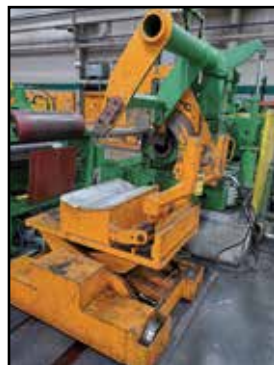
LIGHT GAUGE SLITTING LINE: STAMCO - Pancake Cuts, Non-Plate Strip, .010" - .040" Gauge, .625" - 25.5" Width, 450 FMP, Payoff Arbor - 16" - 20" @16,000-lb., Take-up Arbor - 12.0", 16.0", 20.0" • 520 PIW, PRO-ECO 4 Turnstile Coil Holder, Entry Coil Cart on Track, Payoff Reel Pusher/Tensioner, HORSBURGH & SCOTT Expanded Mandrel De-Coil Reel, STAMCO Breaker, Pinch & Bridle Roll Machines, STAMCO Crop Shear, Out Feed Chip Conveyor, (2) STAMCO Slitting Heads, Tension Roll, Stripper Plate, Loop Tables, Coiling End Reel, End Line Coil Transfer Carriage on Track, (3) Operator Stations, ABB Centerline MCC's, Breaker Cabinet, (5) Transformers, ROCKWELL Automation Drives
