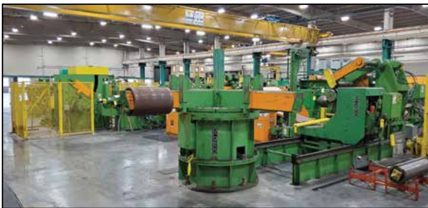
HEAVY GAUGE SLITTING LINE: STAMCO - Pancake Cuts, Non-Plate Strip, .040" - .150" Gauge, .460" - 25.5" Width, 450 FMP, Payoff Arbor - 16" - 20" @16,000-lb., Take-up Arbor - 12.0", 16.0", 20.0" • 520 PIW, PRO-ECO 4 Turnstile Coil Holder, Entry Coil Cart on Track, Payoff Reel Pusher/Tensioner, HORSBURGH & SCOTT Expanded Mandrel De-Coil Reel, STAMCO Breaker, Pinch & Bridle Roll Machines, STAMCO Crop Shear, Out Feed Chip Conveyor, (2) STAMCO Slitting Heads, Tension Roll, Stripper Plate, Loop Tables, Expanding Mandrel Coiling Reel, End Line Coil Transfer Carriage on Track, (3) Operator Stations, ABB Centerline MCC's, Breaker Cabinet, (5) Transformers, ROCKWELL Automation Drives
