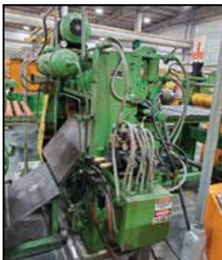
LIGHT GAUGE SLITTING LINE: STAMCO - Pancake Cuts, Non-Plate Strip, .010" - .040" Gauge, .625" - 25.5" Width, 450 FMP, Payoff Arbor - 16" - 20" @16,000-lb., Take-up Arbor - 12.0", 16.0", 20.0" • 520 PIW, PRO-ECO 4 Turnstile Coil Holder, Entry Coil Cart on Track, Payoff Reel Pusher/Tensioner, HORSBURGH & SCOTT Expanded Mandrel De-Coil Reel, STAMCO Breaker, Pinch & Bridle Roll Machines, STAMCO Crop Shear, Out Feed Chip Conveyor, (2) STAMCO Slitting Heads, Tension Roll, Stripper Plate, Loop Tables, Coiling End Reel, End Line Coil Transfer Carriage on Track, (3) Operator Stations, ABB Centerline MCC's, Breaker Cabinet, (5) Transformers, ROCKWELL Automation Drives
