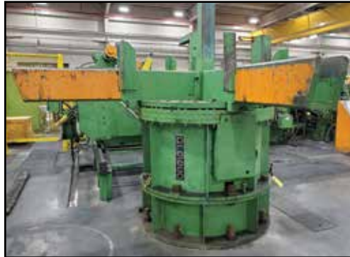
HEAVY GAUGE SLITTING LINE: STAMCO - Pancake Cuts, Non-Plate Strip, .040" - .150" Gauge, .460" - 25.5" Width, 450 FMP, Payoff Arbor - 16" - 20" @16,000-lb., Take-up Arbor - 12.0", 16.0", 20.0" • 520 PIW, PRO-ECO 4 Turnstile Coil Holder, Entry Coil Cart on Track, Payoff Reel Pusher/Tensioner, HORSBURGH & SCOTT Expanded Mandrel De-Coil Reel, STAMCO Breaker, Pinch & Bridle Roll Machines, STAMCO Crop Shear, Out Feed Chip Conveyor, (2) STAMCO Slitting Heads, Tension Roll, Stripper Plate, Loop Tables, Expanding Mandrel Coiling Reel, End Line Coil Transfer Carriage on Track, (3) Operator Stations, ABB Centerline MCC's, Breaker Cabinet, (5) Transformers, ROCKWELL Automation Drives
