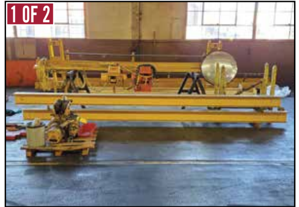
PEC 1/2-Ton x 14' Span Free-standing Bridge Cranes
