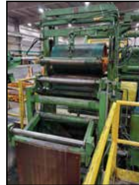
HEAVY GAUGE SLITTING LINE: STAMCO - Pancake Cuts, Non-Plate Strip, .040" - .150" Gauge, .460" - 25.5" Width, 450 FMP, Payoff Arbor - 16" - 20" @16,000-lb., Take-up Arbor - 12.0", 16.0", 20.0" • 520 PIW, PRO-ECO 4 Turnstile Coil Holder, Entry Coil Cart on Track, Payoff Reel Pusher/Tensioner, HORSBURGH & SCOTT Expanded Mandrel De-Coil Reel, STAMCO Breaker, Pinch & Bridle Roll Machines, STAMCO Crop Shear, Out Feed Chip Conveyor, (2) STAMCO Slitting Heads, Tension Roll, Stripper Plate, Loop Tables, Expanding Mandrel Coiling Reel, End Line Coil Transfer Carriage on Track, (3) Operator Stations, ABB Centerline MCC's, Breaker Cabinet, (5) Transformers, ROCKWELL Automation Drives
