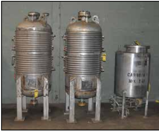
150-Gallon (Est.) 316 SS Jacketed Reactor, 400 PSI
