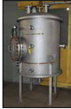
RAS Process Alloy-20 Reactor
