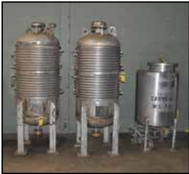
150-Gallon (Est.) 316 SS Jacketed Reactor, 400 PSI
