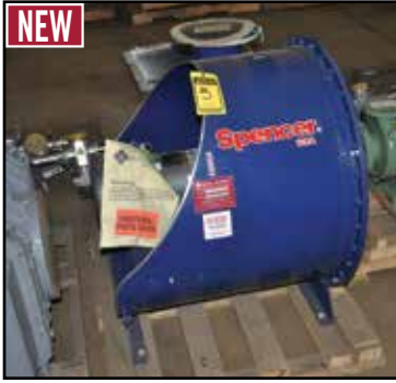
NEW SPENCER G-1205-H MOD 5 HP 3 PH Gas Booster
