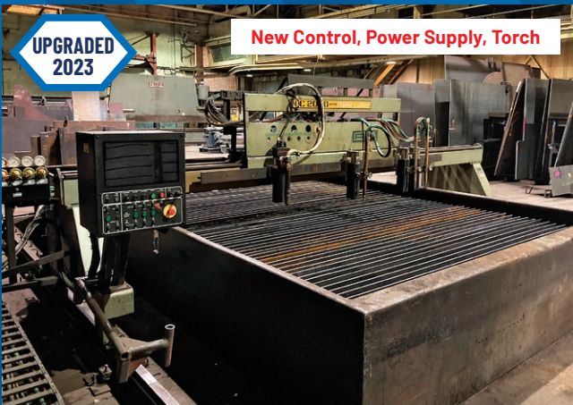
CSI 10' x 25' CNC Plasma Table, Upgraded 2023 at Cost of $150K
