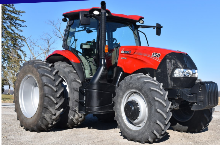
2017 Case IH Maxxum 150 MFWD Multicontroller, Super clean field ready tractor with only 1277 hrs.! autosteer ready, 16 speed power shift with high/low, serial # ZGEE07798, firestone 460/85R 38 rears "Performance 85", axle duals, 540 P.T.O. (interchangeable) 380/85R 28 fronts, (4) S.C.V.'s., fender 3 point, P.T.O. & S.C.V. controls, left hand reverser, new tires, rear duals & spacers, L.E.D.'s (8) 45 Kg front weights, sunroof & sunshade, power beyond hydraulics, 113L/Min CCLS Pump, deluxe radio with Bluetooth, From Ken Shidler
