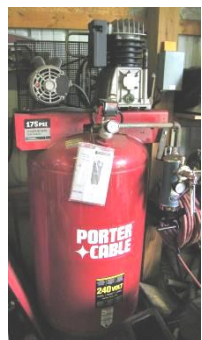
Porter Cable 7 hp, 80 gpl, 175 psi, 240v air compressor,
